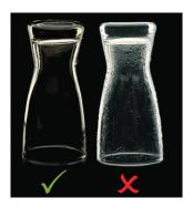
**SHEETING TEST:** A beer clean glass will shed water evenly in unbroken "sheets". On a glass with invisible film, water will break up and form droplets on the surface of the glass.
