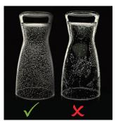
**SALT TEST:** In a beer clean glass, salt sprinkled on the interior of a wet glass will adhere evenly. If not properly cleaned, salt will fall to the bottom or adhere in a random pattern. Salt will not stick wherever a greasy film is present.
